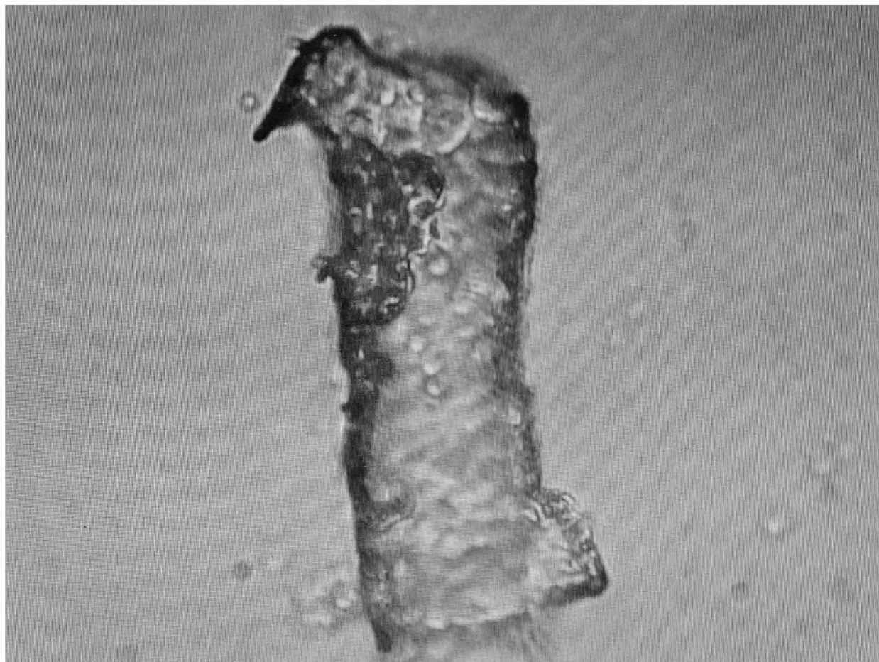
Figure 6 Longitudinally open fiber with broken end and Darpa Hydrogel content balls.
